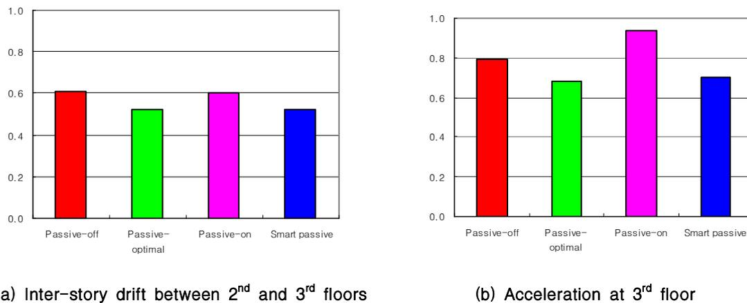
Fig. 9. Comparison of maximum responses normalized by the uncontrolled case
