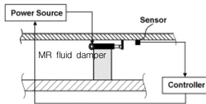
Fig.1. Schematic diagram of an MR fluid damper-based control system
