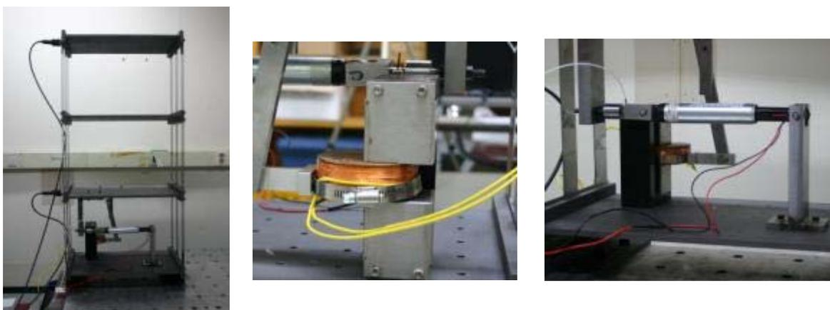
(a) small-scale building model      (b) MR fluid damper with EMI part      (c) EMI part
