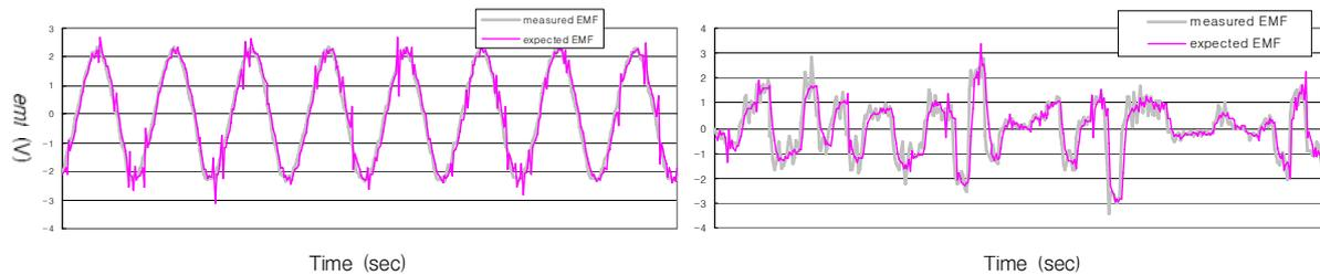
(a) The induced emf under the sinusoidal input      (b) The induced emf under the random input
