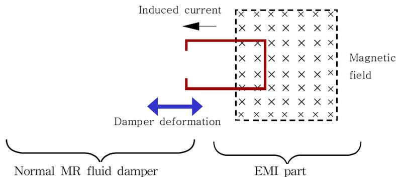
Fig.2. Smart passive control system with MR fluid damper and EMI part
