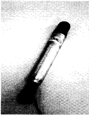
Fig. 4. Magnetorheological (MR) damper
