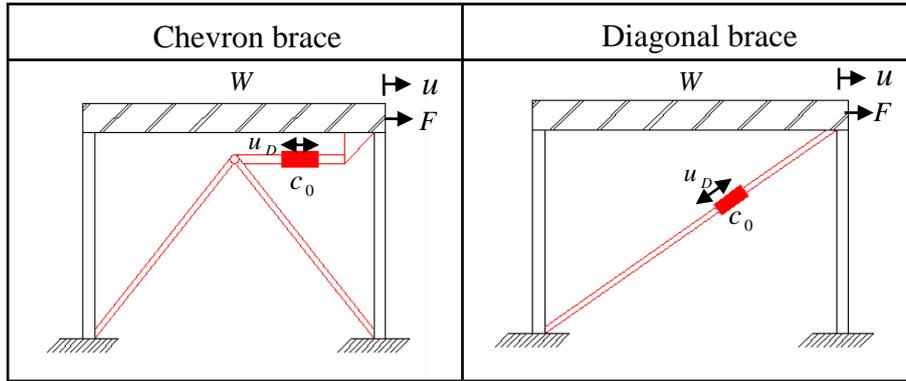
Fig. 1. Illustration of a single-story structure with diagonal and chevron brace.
