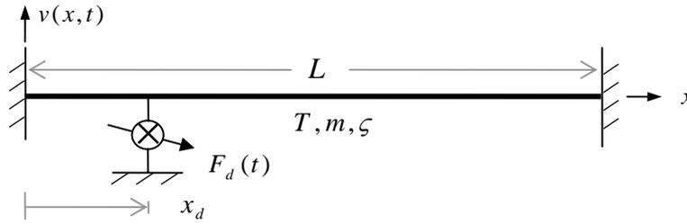
Fig. 5. Cable with attached damper
