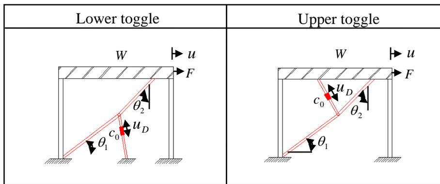
Fig. 2 Illustration of toggle-brace-damper configuration.
