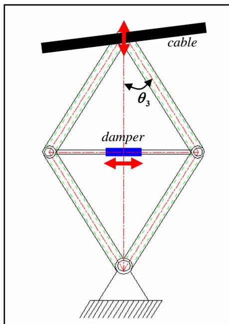
Fig. 4. Illustration of Scissor-Jack-Brace Damper Configuration for stay cable.
