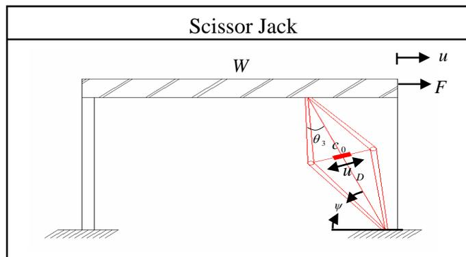
Fig. 3. Illustration of scissor-jack-brace damper configuration.
