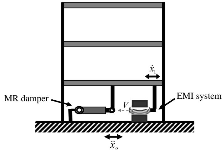
Fig. 1. Schematic of a smart passive system attached to a three-story building
