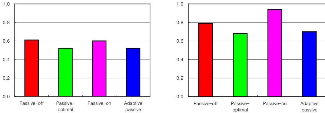
(a) Inter-story drift between 2<sup>nd</sup> and 3<sup>rd</sup> floors (b) Acceleration at 3<sup>rd</sup> floor
