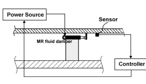
**Figure 1. Schematic diagram of an MR fluid damper-based semiactive control system**
