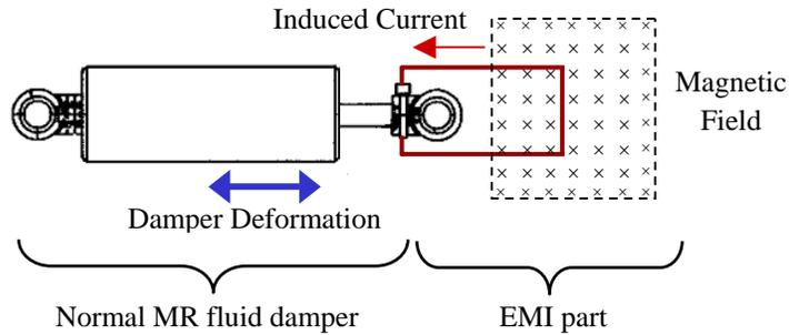
**Figure 2. Proposed control system with MR fluid damper and EMI part**
