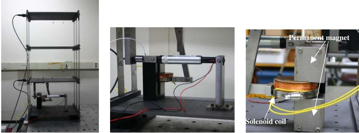
(a) small-scale building model (b) MR fluid damper with EMI part (c) EMI part in detail
