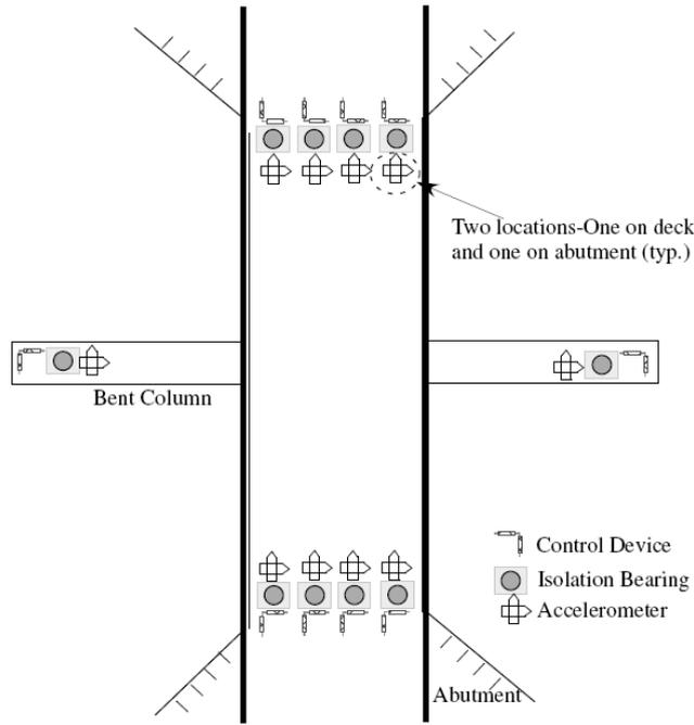
**Figure 1. Locations of control devices and sensors on the bridge**
