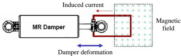
**Figure 2. Schematic model of the MR damper equipped with EMI system**
