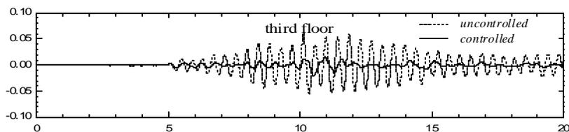
Figure 1. Displacement under Northridge earthquake
