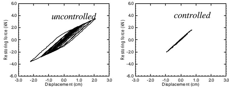
Figure 2. Restoring force vs. displacement under Northridge earthquake
