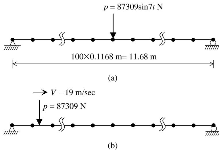
Figure 3.1 Simple span beam: (a) Single input load (sinusoidal load), (b) Multi-input load (moving load)
