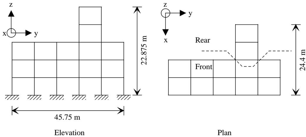
Figure 2.5 Geometry of three-dimensional frame structure
