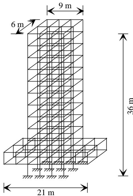
Figure 2.7 Geometry of three-dimensional building structure
