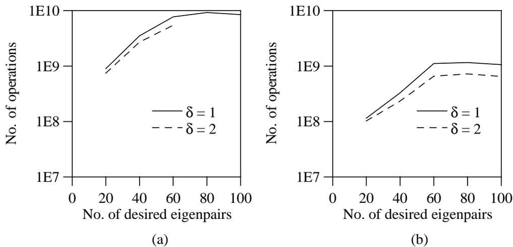
Figure 2.8 Number of operations of three-dimensional building structure: (a) Matrix-powered subspace iteration method, (b) Matrix-powered Lanczos method
