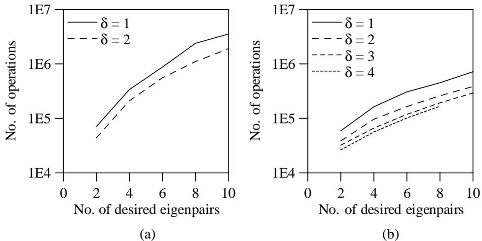
Figure 2.2 Number of operations of simple spring-mass system: (a) Matrix-powered subspace iteration method, (b) Matrix-powered Lanczos method
