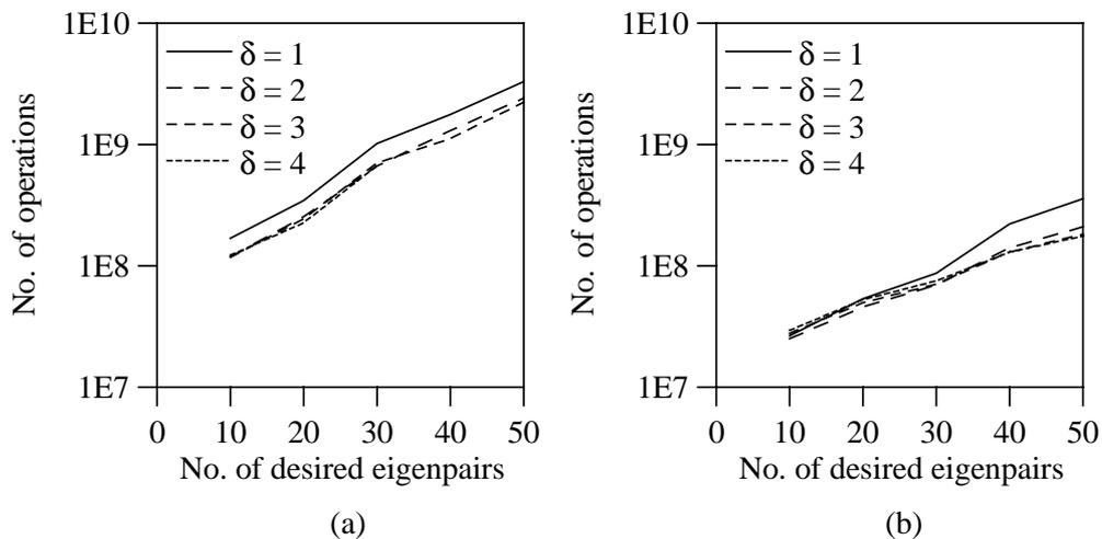
Figure 2.6 Number of operations of three-dimensional frame structure: (a) Matrix-powered subspace iteration method, (b) Matrix-powered Lanczos method
