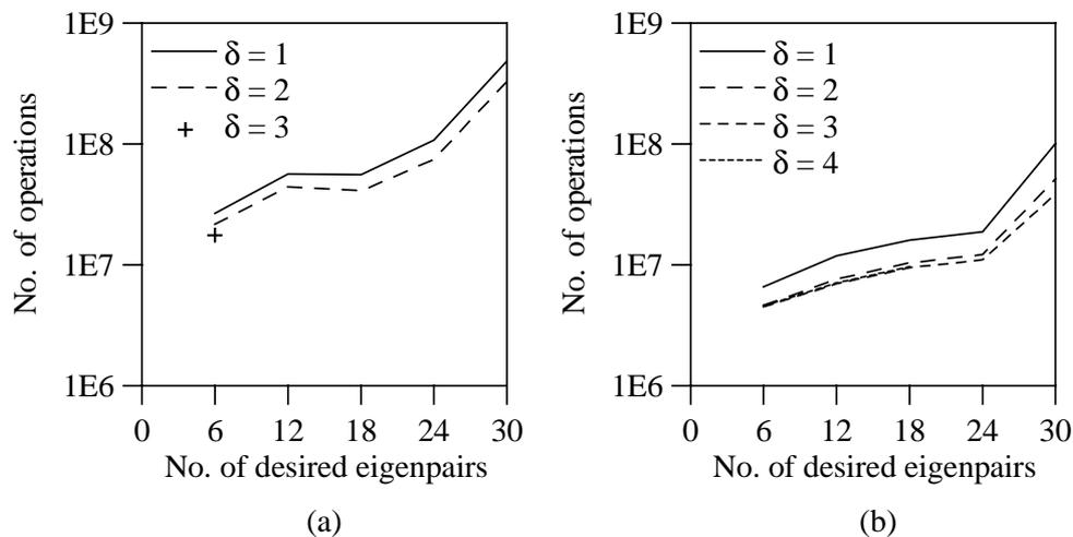
Figure 2.4 Number of operations of plane frame structure: (a) Matrix-powered subspace iteration method, (b) Matrix-powered Lanczos method
