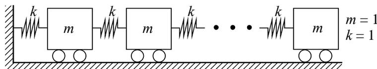
Figure 2.1 Geometry of simple spring-mass system
