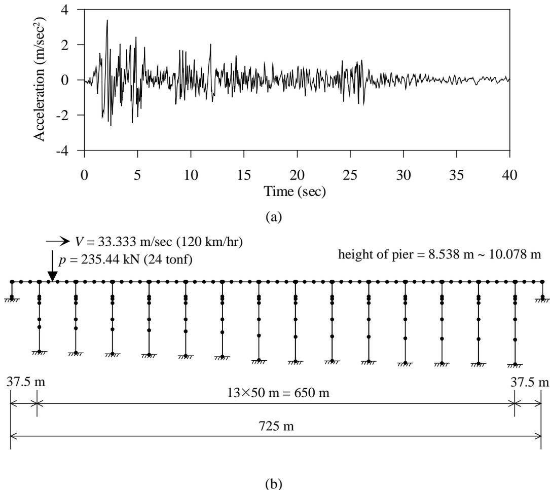
Figure 3.4 Multi-span continuous bridge: (a) Single input load (El Centro earthquake),
